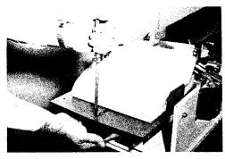
12. Adjust the weight so that it exerts enough force on the wicket to keep it from slipping out from under the lip.
