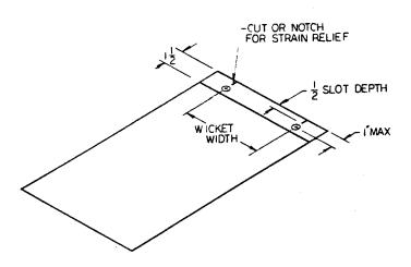
The width of the wicket should never be more than the maximum width of the product to be bagged, and should be centered on the bag. Note: If the wicket were wider than the product you would have to have a wider bag than normally required to handle the same size product.
