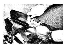
4. Set the width of the funnel arms so that when the funnels are parallel they are the same width and in line with the side guides. A straight edge may be used to make this adjustment.
