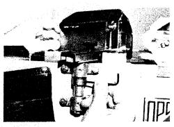
6. If it is necessary to increase the funnel return spring tension, remove the side guard and using a hex allen wrench loosen the spring collar. Rotate the collar until desired tension is reached, retighten the collar and replace the guard.
