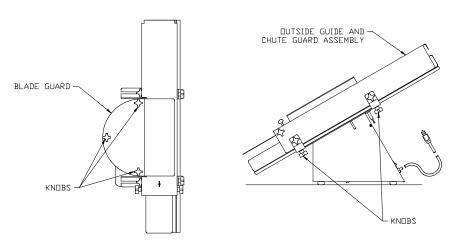
Remove the OUTSIDE GUIDE AND CHUTE GUARD ASSEMBLY by loosening both knobs which secure it in place, and then slide the assembly off the machine and set it aside.
