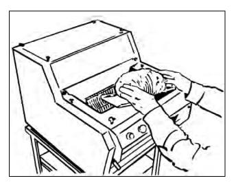
The bagging scoop¢ bread stop is adjustable to accommodate various size loaves. To adjust, apply pressure to the outside edges of the bread stop and slide it along the scoop to the desired position.
