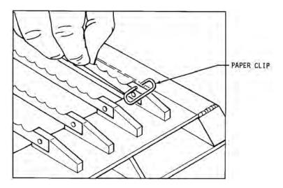
The blades can be removed from the lower blade frame while it is still in the machine. This is done by using a second special blade changing tool. Insert the tool into the blade frame, push the handle toward the feet of the blade frame as shown below. This will reduce the tension on the blade so that it can be carefully removed.
