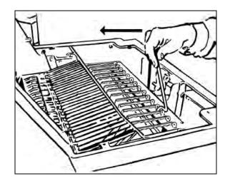
Using the same technique as used on the upper blade frame, replace the knives in the lower blade frame.
