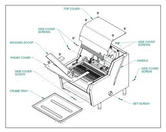
Remove the bagging scoop, the top and front guards by removing the ten knobs which secure them in place, also remove the crumb tray. Remove the handle by loosening the set screw which holds the handle after which it can be slid out of the hub. The cover can then be removed by first removing the six slotted head screws which secure it in place. See the above illustration to see their approximate locations.
