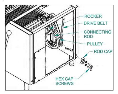
After replacing the belt reattach the connecting rod making sure to place the connecting rod as perpendicular as possible to the rockercs main shaft. Retighten the rod capcs bolts securely. Tighten the belt as described in the Weightening the Belt+section of this manual and then replace the top cover.
