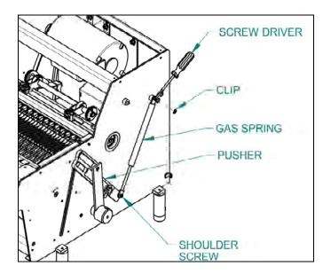
Install a gas spring by first attaching the lower end of the spring to the pusher arm with the shoulder screw.
