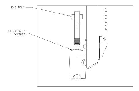
When replacing the eye bolts turn them clockwise until moderate pressure is required to close the cam. If the cam is to easy to close rotate the eye bolt a half turn more in the clockwise direction and try to reinstall the cam. Repeat these partial rotations until moderate pressure is required to close the cam. If the cams are either difficult or impossible to close, rotate the eye bolt a half turn in the counter clockwise direction. Repeat until the cams can be closed using moderate pressure.
