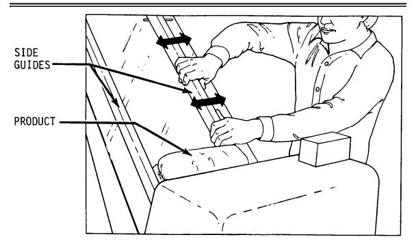
Adjusting the Outfeed Side Guides on a Standard Outfeed Table
