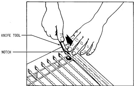
The new knife can be installed by reversing the removal procedure. A paper clip can be used to hold the knife in position on the lower pin to ease installation. See the illustration below.
