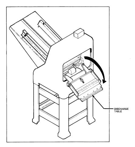
Always start by removing the discharge side blade frame first. Both blade frames should be removed from the discharge side of the machine. You should remove the discharge side blade frame completely from the machine before starting on the infeed side blade frame. However each is removed using similar procedures.
