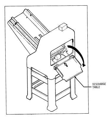
Always start by removing the discharge side blade frame first. Both blade frames should be removed from the discharge side of the machine. You should remove the discharge side blade frame completely from the machine before starting on the infeed side blade frame. However each is removed using similar procedures.
