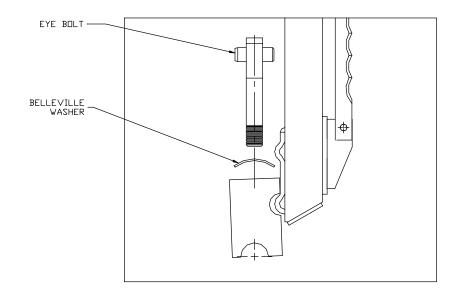
When replacing the eye bolts turn them clockwise until moderate pressure is required to close the cam. If the cam is to easy to close rotate the eye bolt a half turn more in the clockwise direction and try to reinstall the cam. Repeat these partial rotations until moderate pressure is required to close the cam. If the cams are either difficult or impossible to close, rotate the eye bolt a half turn in the counter clockwise direction. Repeat until the cams can be closed using moderate pressure.
