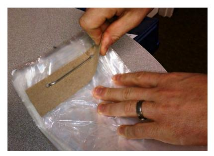
5. Select the appropriate hole spacing in which to place the wicket of bags by lifting the spring hold down and inserting the wicket into the holes.
