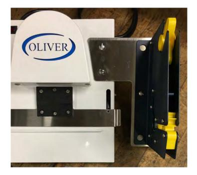
4. Before placing the bags on the unit, remove the cardboard backing from the top side of the wicket.
