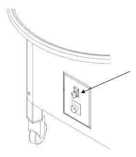
Balance the rate at which the table turns and is loaded and unloaded to avoid overfilling the tabletop.
