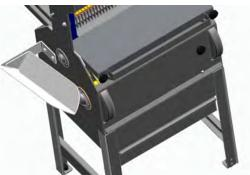
Installing the Front Bagging Scoop (as applicable)
