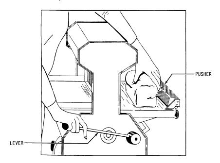
While continuing to hold the lever down with the right hand move the left hand to the discharge side of the machine and pull the motor starting knob, see next illustration. Allow the right hand to raise slowly with the lever until the loaf contacts the slicer blades. After the knives have pierced the crust remove your right hand from the lever allowing the pusher to move the loaf through the knives.
