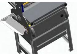
Installing the Front Bagging Scoop (as applicable)
